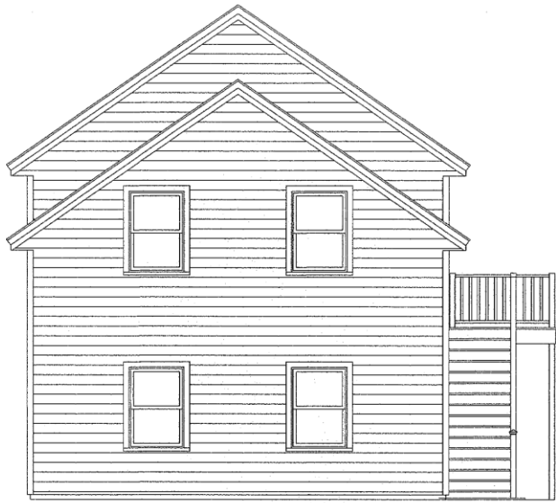
FRONT EXTERIOR ELEVATION SCALE : 1/4" = 1'-0"
